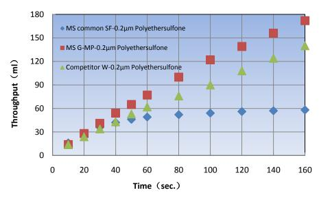
Dynamic throughput via 25mm syringe filters was tested at 10psi with 2.5% TSB (Trypticase Soy Broth)
